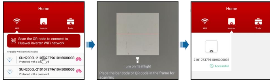
Figure 7-6 Scanning the QR code to connect the mobile phone to the SUN2000L directly
